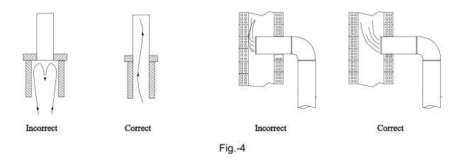
*e) It is very important* to ensure that the joints of the pipes are well sealed to avoid possible cracks through which air may enter.
