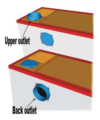
The cooker is supplied with smoke outlet the ring installed on the upper outlet. In order to change the ring from the top to the back release the four outlet. screws that attach it to the hob, remove the cover on the back outlet and install the ring. Place the ring on the back outlet and the cover on the top outlet.
